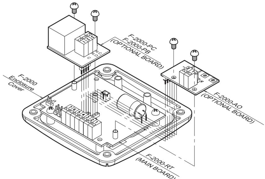
1.3 Model RT Circuit Board Wiring
