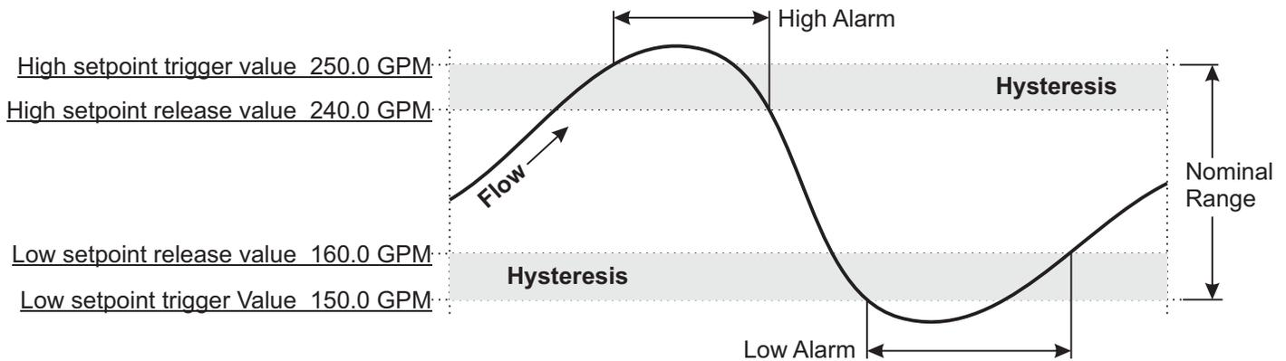
Note: If the relay flickers on and off due to unstable flow, readjust the release value to increase the amount of hysteresis.
