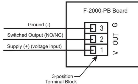
Output Type: Non-Isolated contact closure switch, NO / NC
