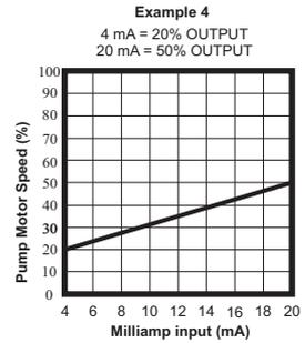
**Note:** Pump can be set from 0 - 100% motor speed in any input mode; however, actual working range of pump is from 10 - 100% motor speed, therefore motor may not start to rotate below 10% motor speed.
