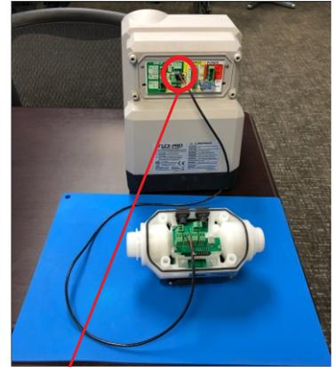
**Step 1.** Connect 4.7k Ohms resistor from PIN 1 to PIN 2 of the terminal marked T4 on the ProSeries pump wiring terminal.
