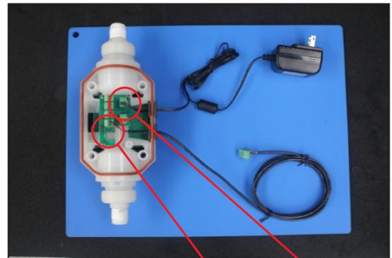
In this example the user has wired both Power and 4-20mA Out.
