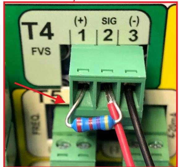
**Step 2.** Trim the bare and connect the RED WIRE to PIN 2 (SIG) and the BLACK WIRE to PIN 3 of the terminal marked T4
